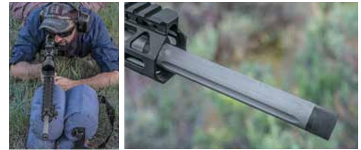
The 20-inch barrel comes threaded for suppression, and the flutes reduce weight and cooling time.
